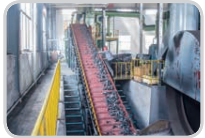
④ Shot Blasting
